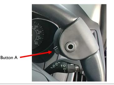
The button for 'Front wiper' can be used to operate up to three functions. They are 'Short wiping', 'Increase wiper speed' and 'Washer'.
